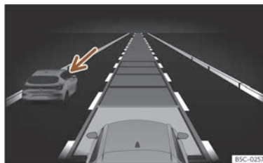
Fig. 134 On the instrument cluster screen: ACC active, vehicle detected on the left.
