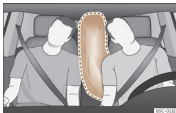
Fig. 33 Fully inflated central airbag (deployment zone).
