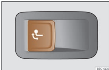
Fig. 196 Left side of the luggage compartment: button to unlock the tow hitch.
