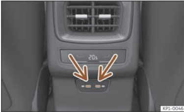
Fig. 174 Rear centre console: USB connectors with power socket function.
