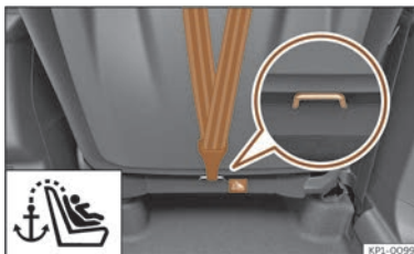
Fig. 44 Rear of front passenger seat backrest: Top Tether belt anchor (not available on all markets).
