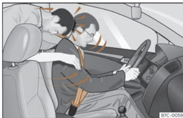
Fig. 22 Any rear seat occupants not wearing a seat belt may be thrown forward violently, hitting the driver who is wearing the seat belt.
