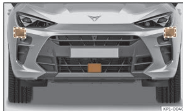
Fig. 123 On the front bumper: front and side radar sensors.
