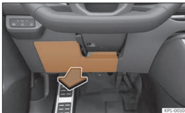
Fig. 215 On the dashboard on the driver side: lid of the fuse box.
