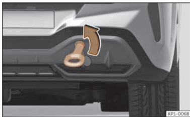
Fig. 214 Right side of the rear bumper: towline anchorage screwed in.
