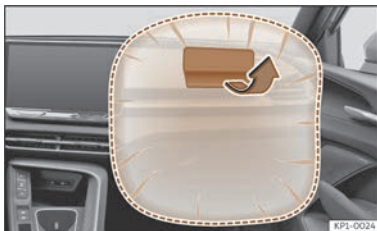
Fig. 29 Front passenger airbag located in dash panel.
