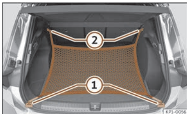
Fig. 191 In the luggage compartment: rings ① and hooks ② for attaching the net bag.
