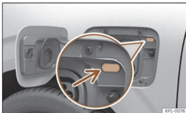
Fig. 61 Behind the battery charging socket cover: charging process indicator.
