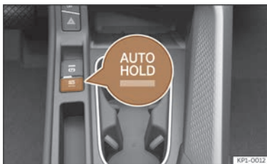
Fig. 148 In the lower part of the centre console: Auto Hold function button.
