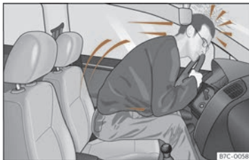
Fig. 20 A driver not wearing a seat belt may be thrown forward violently.
