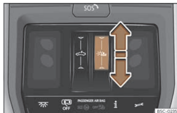
Fig. 91 On the headliner: operate the sun blind.
