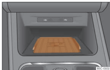
Fig. 180 On the centre console: pad for the mobile phone connection.
