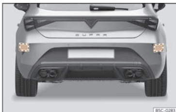
Fig. 133 Rear view of the vehicle: radar sensor areas.
