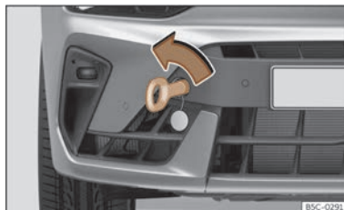
Fig. 220 Right side of the front bumper: towline anchorage screwed in.
