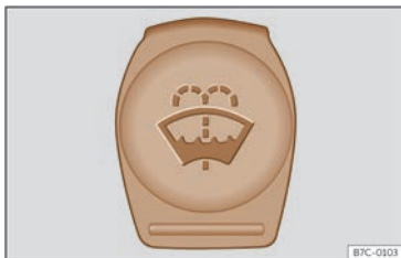
Fig. 232 In the front compartment: blue cap of the windscreen washer reservoir.
