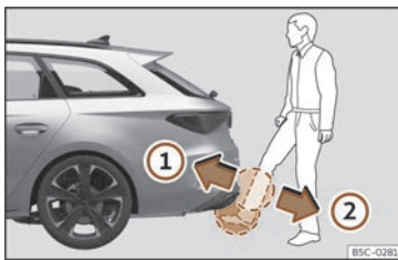
Fig. 85 Rear lid with sensor-controlled opening (Easy Open).
