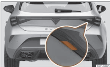
Fig. 82 Rear lid: opening from the outside.
