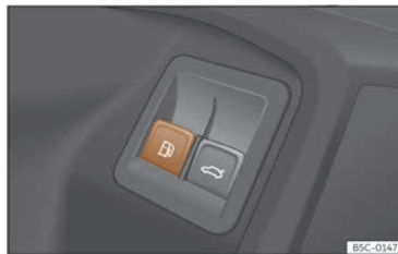
Fig. 210 Driver's door: tank flap release.
