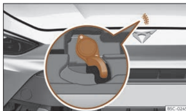
Fig. 227 Lever under the bonnet.
