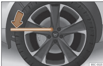
Fig. 248 Tyre change: loosen the wheel nuts.
