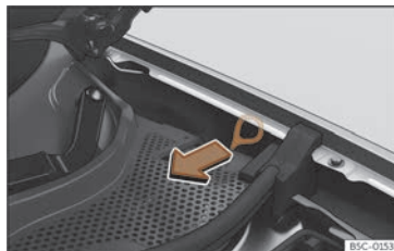
Fig. 65 Between the left wing panel and the engine bonnet hinge: Charging connector manual release mechanism puller.
