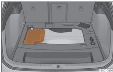
Fig. 238 Hybrid vehicles (PHEV): location of the battery in the luggage compartment
