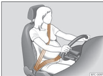
Fig. 25 Position of seat belt during pregnancy.
