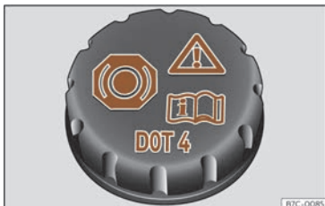
Fig. 231 Front compartment: brake fluid reservoir cap.
