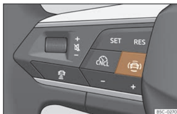
Fig. 129 Left side of the multifunction steering wheel: button for driver assistance systems (depending on the version).
