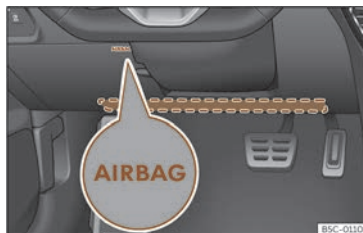
Fig. 35 On the driver side: location of the knee airbag.
