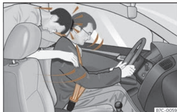
Fig. 21 Any rear seat occupants not wearing a seat belt may be thrown forward violently, hitting the driver who is wearing the seat belt.
