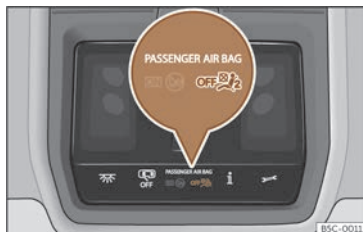
Fig. 29 On the roof console: passenger airbag deactivation control lamp.
