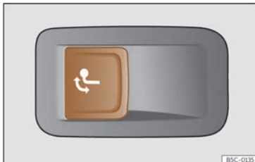
Fig. 205 Left side of the luggage compartment: button to unlock the tow hitch.
