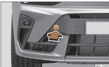
Fig. 219 Front bumper on right: remove the lid.
