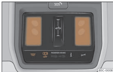
Fig. 109 Detail of headliner: front interior lighting.
