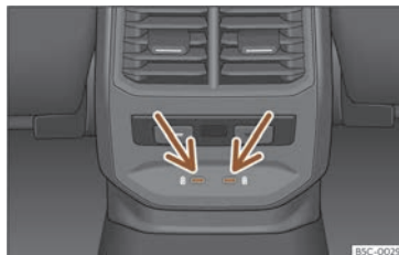
Fig. 174 Rear centre console: USB connectors with power socket function.
