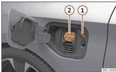
Fig. 60 Behind the battery charging cover on the front left-hand side: Charging socket
