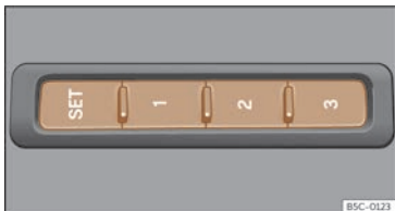
Fig. 103 On the outer side of the driver's seat: memory buttons.
