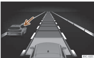
Fig. 141 On the instrument cluster screen: ACC active, vehicle detected on the left.
