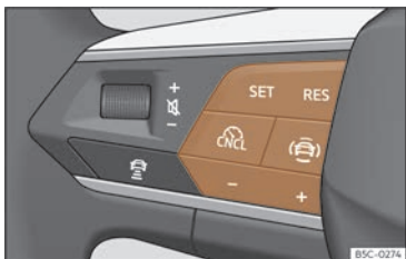
Fig. 137 On the multifunction steering wheel: buttons to control the speed limiter.
