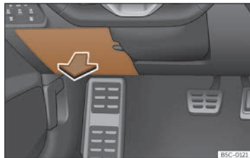
Fig. 223 On the dashboard on the driver side: lid of the fuse box.
