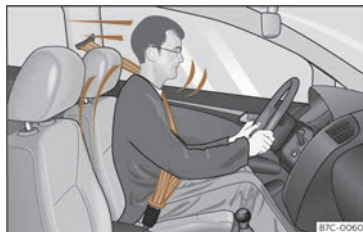
Fig. 18 Drivers with properly worn seat belts will not be thrown forward in the event of sudden braking.
