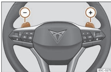
Fig. 127 Steering wheel: automatic gearbox levers
