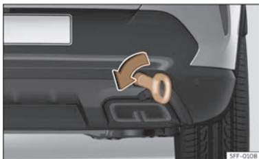
Fig. 216 Right side of the rear bumper: towline anchorage screwed in.
