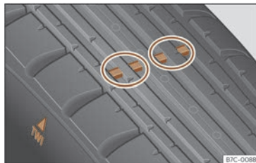
Fig. 236 Tyre profile: tread wear indicators.
