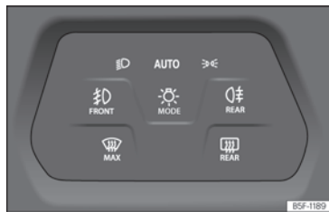
Fig. 107 Instrument panel: light panel.
