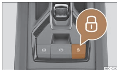
Fig. 79 On the centre console: central locking button
