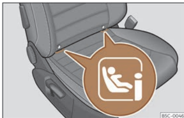
Fig. 41 Front passenger seat: location of the i-Size securing rings.
