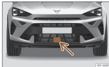
Fig. 131 On the front bumper: radar sensor.
