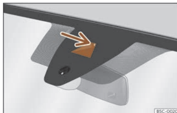
Fig. 133 On the windscreen: field of vision of the Lane Assist system camera.
