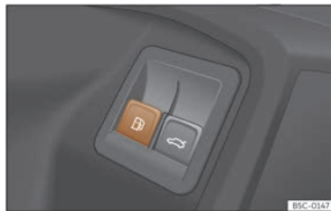
Fig. 204 Driver's door: tank flap release.
