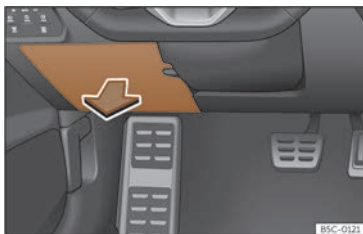
Fig. 217 On the dashboard on the driver side: lid of the fuse box.
