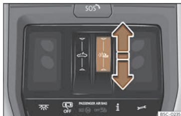
Fig. 92 On the headliner: operate the sun blind.
