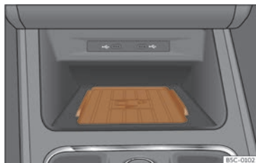
Fig. 184 On the centre console: pad for the mobile phone connection.
