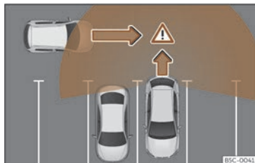
Fig. 169 Diagram of the parking assistant: detected area around the vehicle that is driving off.
