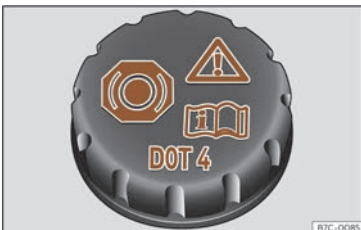
Fig. 225 Front compartment: brake fluid reservoir cap.
