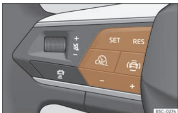
Fig. 138 On the multifunction steering wheel: buttons to control the speed limiter.
