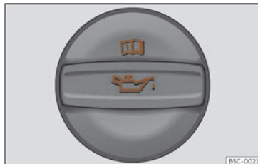
Fig. 231 Oil filler cap cover in the engine compartment.
