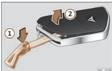
Fig. 74 Vehicle key: open the battery compartment cover.
