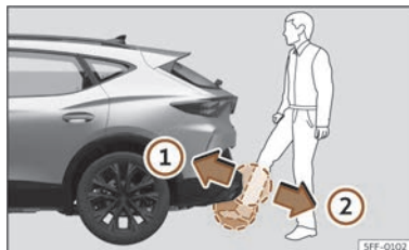
Fig. 86 Rear lid with sensor-controlled opening (Easy Open).
