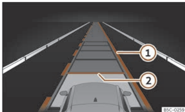
Fig. 148 On the instrument cluster display: display of active regulation (schematic representation).
