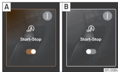
Fig. 124 In the infotainment system: Start-Stop system (accessible from different infotainment menus).
