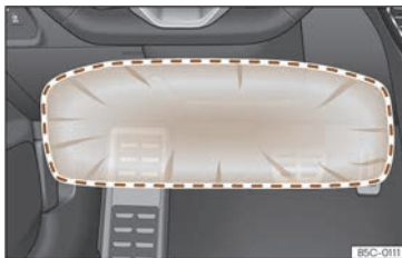
Fig. 36 On the driver side: action radius of the knee airbag.
