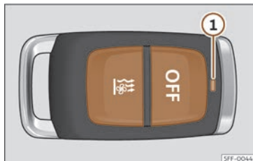
Fig. 120 Auxiliary heating: radio remote control.
