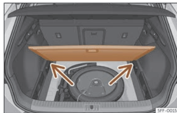
Fig. 190 Variable boot floor: tilted position.
