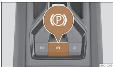
Fig. 155 Centre console, lower part: electronic parking brake button.
