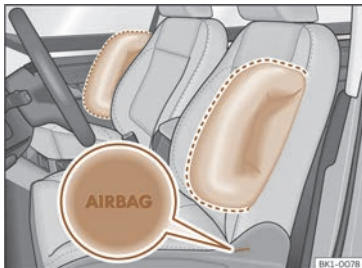
Fig. 32 Driver's seat and passenger seat side airbags.
