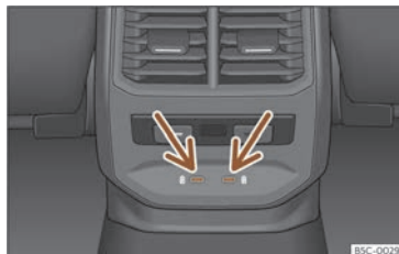
Fig. 178 Rear centre console: USB connectors with power socket function.
