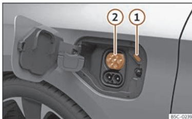
Fig. 60 Behind the battery charging cover on the front left-hand side: Charging socket
