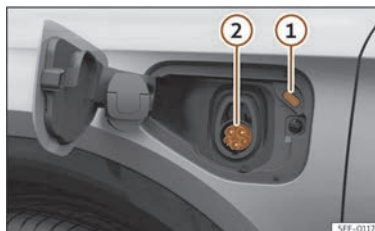
Fig. 61 Behind the battery charging cover on the front left-hand side: Charging socket (depending on the market).
