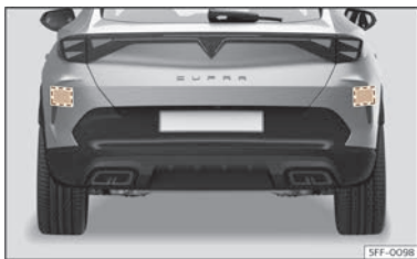
Fig. 134 Rear view of the vehicle: radar sensor areas.
