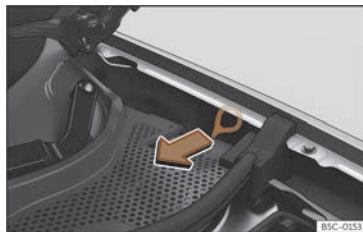
Fig. 66 Between the left wing panel and the engine bonnet hinge: Charging connector manual release mechanism puller.
